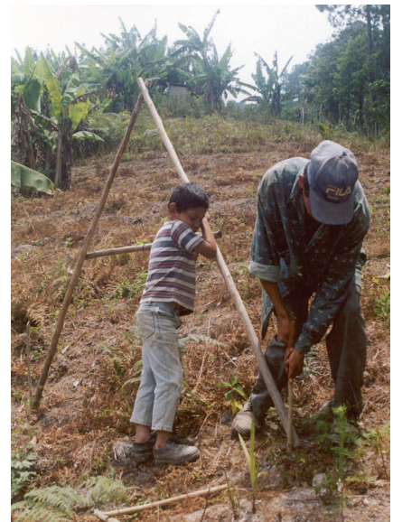
Children learn from their parents how to use an “A” frame to lay out contours in order to manage water and conserve soil.
